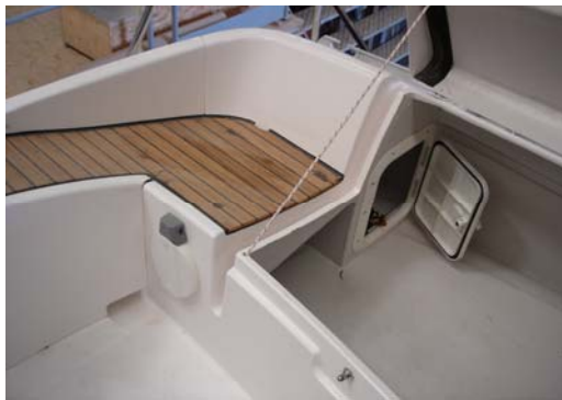
Manual bilge pump in port side cockpit compartment
