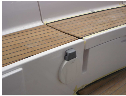
Manual bilge pump on Port side of cockpit
