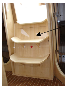
Engine compartment fire-extinguisher hose hole Location between main companionway steps
