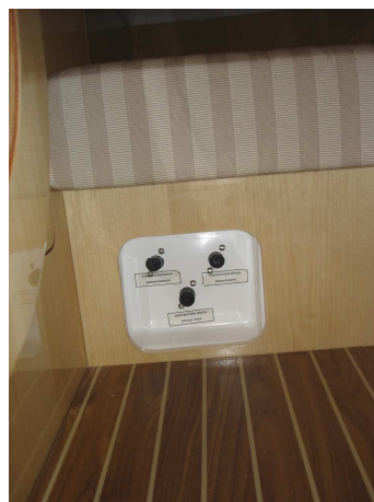
Location of isolators in aft port cabin
