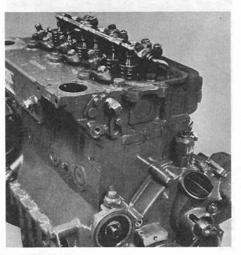
3. Remove the fuel filter, the oil filter, the feed-pump, the thermostat housing and the exhaust elbow. Also remove the sea-water pump with its attachment tubes.
