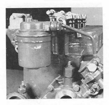
18. Install the feed pump and the fuel filter. Also install the thermostat housing with the thermostat. NOTE! Do not forget the lifting eyelet between the fuel filter and the thermostat housing.
