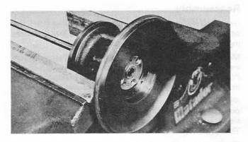
Unfasten the four screws which hold the compression bearing (8). Using a small copper mandrel, tap out the compression bearing and the bushing (9). Then remove the circlips (10) inside the bearing housing and remove the two bearings (11).
