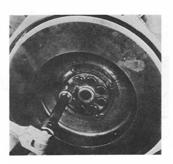
11. Remove the outer flywheel housing, the flywheel and the inner flywheel housing.
