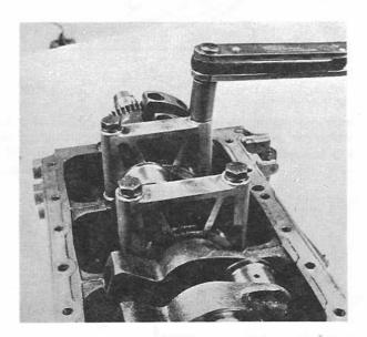
2. Oil the cap bearing halves and install them. Install the caps in accordance with the marking in the block (2001 has no intermediate bearing). If an arrow is cast, it shall point towards the oil dipstick. Tightening torque for the main bearings: 1st tightening 20 Nm (2 kpm) (14.7 ft.lbs), 2nd tightening 60 Nm (6 kpm) (44.2 ft.lbs). Turn the engine.
