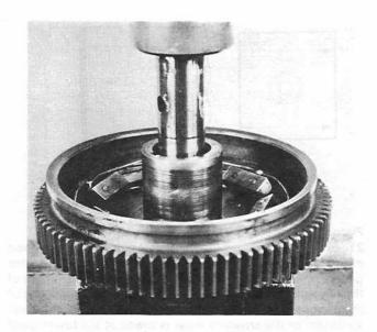
19. Place a support under the camshaft gear and use a hydraulic press to remove the gear.
