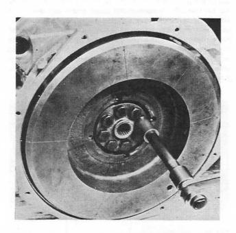
6. Replace the O-rings and install the flywheel housing. Tightening torque 25 Nm (2,5 kpm) (18.4 ft.lbs). Install the flywheel. Tightening torque 65 Nm (6,5 kpm) (48.0 ft.lbs).
