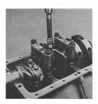
13. Remove the connecting rod bolts and remove the connecting rods and the pistons. The connecting rod and the connecting rod cap are marked with figures.
