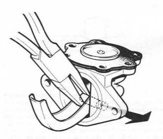
15. Use a suitable pair of pliers and remove the pump lever shaft. Pull out the lever and the diaphragm.
