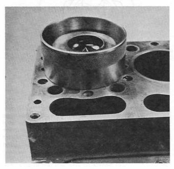
3. Turn the piston rings so that the gaps are offset in relation to each other. The piston crown is marked with an arrow that points towards the belt pulley. Use installation ring 884813-7. Fit the caps with the marking aligned with the crankshaft's marking. The crankshaft can be turned in any direction towards the piston.
