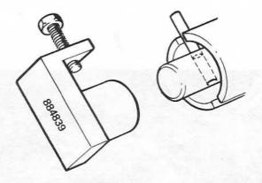
**7B.** Install a new sealing ring for the camshaft in the transmission housing, using mandrel p/n 884838. The sealing lip with the spring is to be turned towards the engine. Press in the sealing ring from the outside until the mandrel "bottoms" against the housing. Install a new O-ring in the oil channel in the block (3 fig. 7A).
