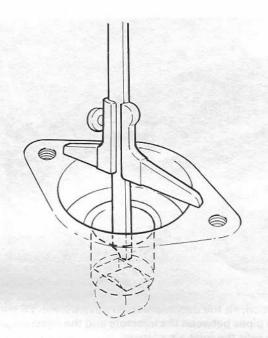
C. Turn cylinder no. 1 to it's injection position. Place the guide pin (2) in the setting-disc's hole marked cyl. 1. Turn the crankshaft a little against the normal direction of rotation and thereafter in the normal rotation direction until the setting-disc's guide pin (2) goes in the timing cover's hole. Measure using a caliper the distance between the cylinder block and the roller lifter's edge (do not measure on the roller).
