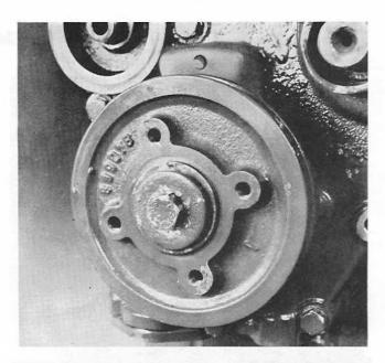
10. Insert the key for the pulley in the crankshaft and install the pulley. Tightening torque 40 Nm (4,0 kpm) (29.5 ft.lbs).
