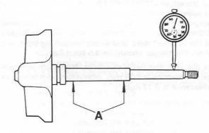
Place the shaft on two supports, which should be under the bearing recesses, and check the throw at the end of the shaft. The maximum permissible throw is 0.011 mm.
