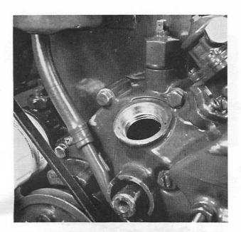
23. Fill up with lubricating oil to the correct level. Regarding quantity and quality, see under "Technical Data".
