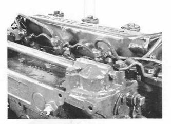
21. Fit the valve cover using a new gasket. Make sure that the round hole for the crankcase ventilation is in the right position. Fit the decompression device lever. Fit the pressure pipes between the injectors and the injection pumps. Also refit the inlet air silencer.
