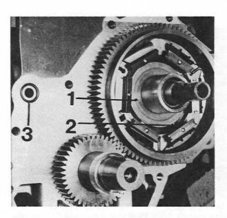
7A. Heat the camshaft gear wheel to a temperature of approx. 150°C (302°F) and use a suitable sleeve to install it. Check to make sure that the gear wheel "bottoms" on the camshaft. Install the camshaft and make sure that the markings on the camshaft gear wheel and on the crankshaft gear wheel coincide. Put the washer (1) on the hub of the camshaft gear wheel. Check that all weights are pressed in so that the tabs (2) are inside the washer.
