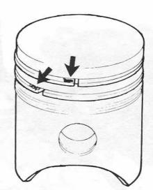
24. Use piston ring pliers to install the piston rings. The marking of the rings (TOP or the mark of the manufacturer) must be turned upwards. The height of the upper compression ring: 1,75 mm (.068898 in.) The height of the lower compression ring: 2,00 mm (.07874 in.). Turn the piston rings so that the gaps are turned 120° from each other.
