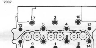
12. Tighten the two guide screws p/n 884840 in the block and install the cylinder head gasket with the marking "Top" facing upwards. Install the cylinder head.
