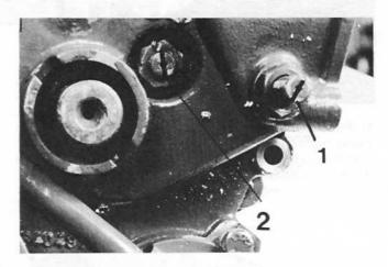
8. The max.-volume-screw (1) and the max.-rev-screw (2) are set by Volvo Penta and must never be changed since this will affect the engine output.
