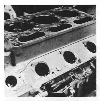
5. Remove the fuel injection pumps. Mark the pumps to ensure installation in the same cylinders from which they were removed. Take care of the shims. Remove the screws on the side of the engine block and lift out the pump lifters.
