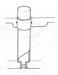
9. Replace the O-ring, sealing off between the sleeve and the cylinder head. Dip the new O-ring in soap-water in order to facilitate the installation. Oil the new injector sleeve and install it, using special tool p/n 884557. Knock down the sleeve until it bottoms.
