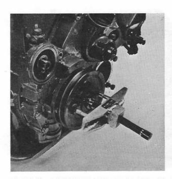
Remove the pulley center bolt and pull off the pulley using puller p/n 9992265. Place a protection pad between the puller and the crankshaft to avoid the crankshaft being damaged.
