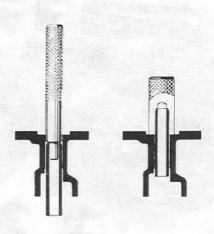
3. Use mandrel p/n 5218 to press out the valve guides. Oil the new valve guides externally and use mandrel p/n 884559 to install them. Press down the mandrel all the way down to the cylinder head. Ream the valve guides if necessary.
