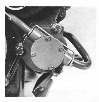
19. Install the sea-water pump and the cooling water pipes.
