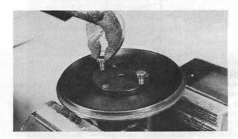
Dismantle the turbine shaft (4) and the heat shield. If the turbine shaft sticks, tap the end gently with a wooden hammer. Unfasten the three screws which hold the cover (3) and screw two M5 screws into the cover. Then lift it up. Take the oil deflector (7) out of the cover.
