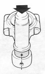
26. Check the connecting rod bushings by using the gudgeon pin as a gauge. There must be no play. If the bushings must be replaced, use a suitable mandrel for the removal and installation. Make sure to install the bushing with the oil hole coinciding with that of the connecting rod. Ream the new bushings. The fit is correct when an oiled gudgeon pin by its own weight can slowly slide through the bushing.
