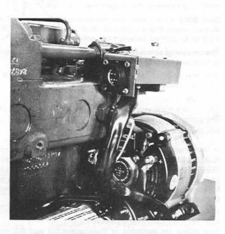
22. Install the starter motor, the alternator and the alternator V-belt. Also install the electrical distribution box and hook-up the cable harness.
