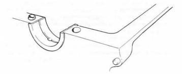
1. Heat the crankshaft gear wheel to approx. 150°C (302°F) prior to the installation. Place the key in the key-way of the crankshaft and press on the gear wheel. Oil the new main bearing halves (with oil hole) and install them in the block. Put in the crankshaft. NOTE! The main bearing shell at the flywheel also functions as a thrust-bearing.
