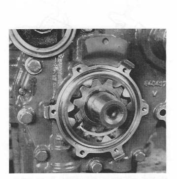
Install the oil pump's gear wheel according to the marks (from the disassembly). Insert a new O-ring in the timing gear cover. Oil the gear wheel and fit the cover using a new sealing ring.
