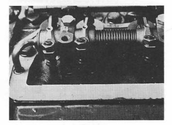
13. Install the push rods and the rocker arm bridge, push on new rubber rings to the oil pipe which is fitted at the same time as the rocker arm bridge.
