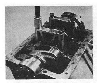
14. Remove the main bearing caps. The main bearing caps are marked with a figure. The corresponding figure is punched into the block. Lift out the crankshaft. On later engine versions an arrow is cast in the separate main bearing caps (2002, 2003). The arrow is to point towards the dipstick.
