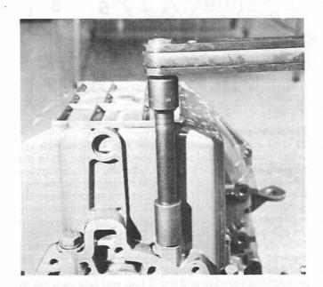
4. Install the main bearing halves in the oil pan and coat the edge of the oil pan with thin layer of sealing compound p/n 840879. Install the oil pan and tighten the oil pan screws and the main bearing screws alternatingly to 20 Nm (2,0 kpm) (14.7 ft.lbs.) and then the main bearing screws to 60 Nm (6,0 kpm) (44.2 ft.lbs.).
