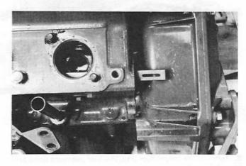
Remove the control rod. Start by removing the plug at the rear of the block and the two screws on the pump plane, holding the control rod.
