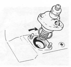
On later version engines an O-ring has been introduced as a seal between the injection pump and the block. Only so-called hard shims may be used on these engines when shimming. Hard shims are available in thicknesses of 0.2 mm (0.0079 in), 0.3 mm (0.0118 in), 0.6 mm (0.0024 in) and 0.9 mm (0.0354 in).
