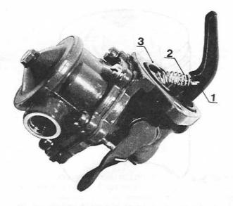
16. Clean the pump housing carefully and replace worn parts. Install the diaphragm and the lever on the diaphragm shaft. Then insert the shaft and tighten it with the screw. Assemble the two housing halves and install the attachment plate (1). Then install the spring (2) and the Oring (3).
