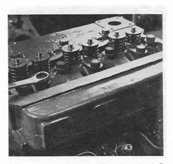
4. Remove the valve bridge and lift out the push rods. Remove the rubber rings for the oil pipe. Remove the cylinder head and the valve lifters. Put the lifters on a rack in consequtive order. NOTE! The cylinder head bolts are phosphatised and must not be cleaned with a steel brush.
