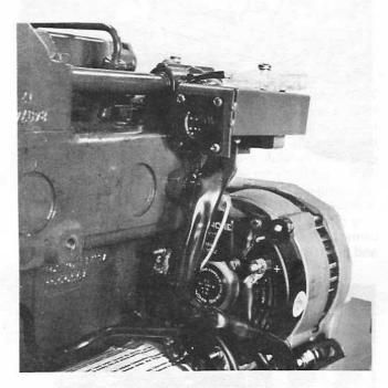
Remove the alternator, the tensioner bracket and the starter motor. Remove the connections from the electrical distribution box from the engine and remove the box and the wire harness.
