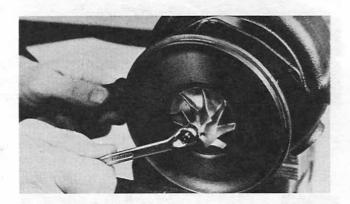
Make line-up marks between the turbine housing, the bearing housing and the compressor housing. Dismantle the compressor housing (1). Unscrew the left-hand threaded nut which holds the compressor wheel, using dollies on the turbine shaft. Remove the compressor wheel (2) and dismantle the turbine housing (3).
