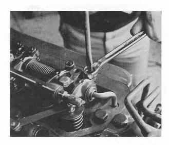
14. Valve clearance cold/warm engine 0.30 mm (.01181 in.). Turn the engine in the direction of rotation until the valves in one cylinder are "rocking". Then turn the engine one turn more and adjust the valves for this cylinder. Repeat the procedure for the remaining cylinders.
