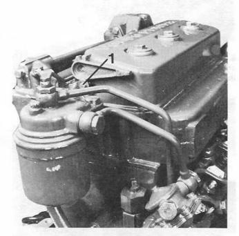
2. Remove the return fuel line, the fuel pressure lines and the inlet air silencer. Install protection caps on the fuel injection pumps and injectors. Remove the screw holding the lever of the decompression device (1) and pull out the lever. Remove the valve cover.
