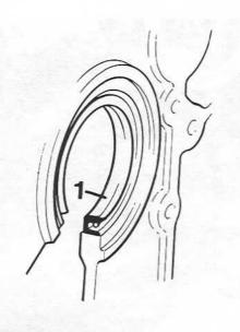
5. Replace the flywheel housing sealing (1). Smear sealing compound (p/n 840879) on the edge between the flywheel housing and the sealing. NOTE! The sealing lip with a spring shall be turned towards the engine. Make sure that the sealing is installed in accordance with the picture.
