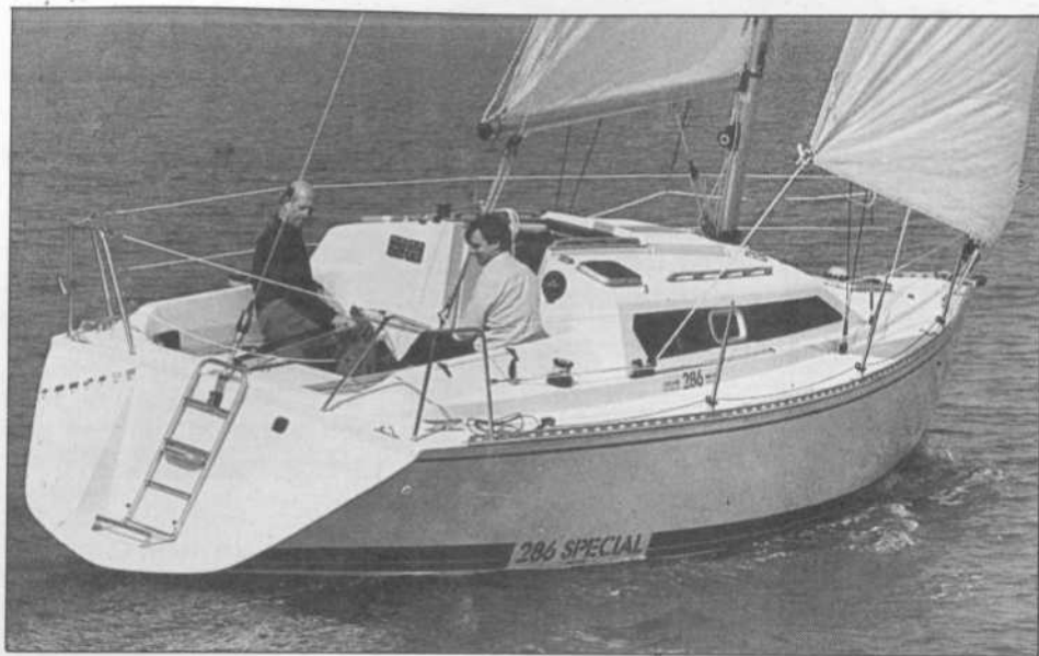
This Gilles Vaton-designed yacht has a fully radiused stem and a distinctive transom
