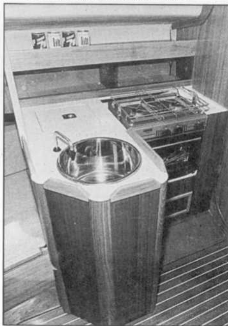
Simple but well-designed galley. L-shaped, positioned just forward of the head
